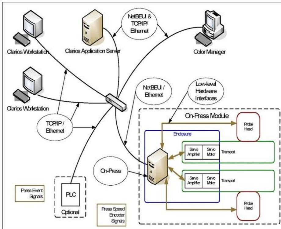
Fig. 5. The architecture of the Inline control system.
