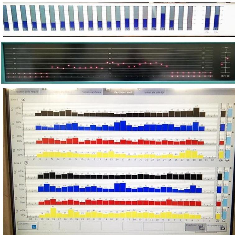
**Fig. 9.** Ink keys opening on different printing presses. a – New digital visual system, b – Old LED graphical system, c – IDC Color Console.
