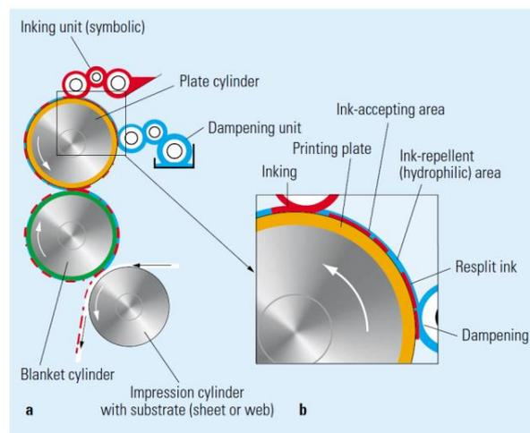
**Fig. 1.** Components of a printing unit.
