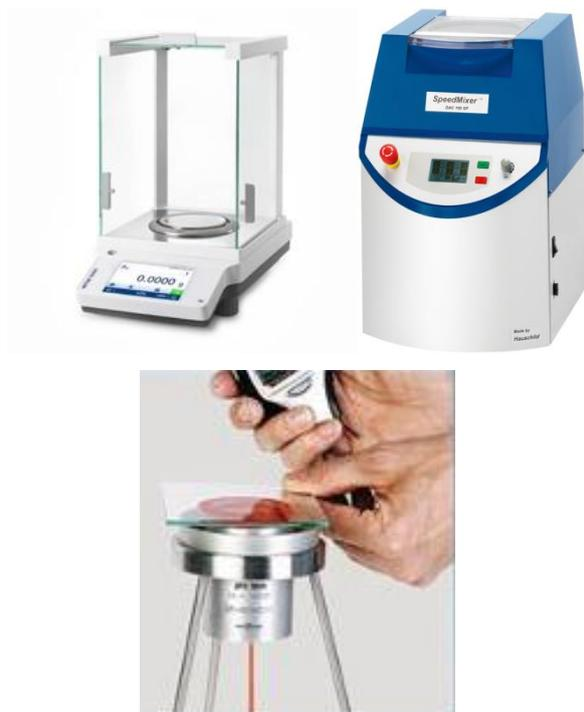
**Fig. 3. Operation of analytical balance, ink speed mixer and flow cup.**
