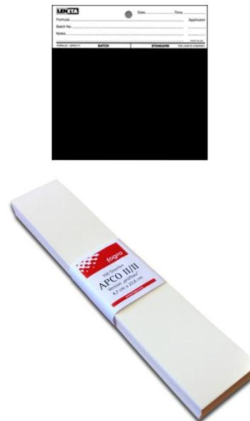
**Fig. 4. Reference Substrates – Leneta and APCO II/II (alternatiely IGT CT2846).**
