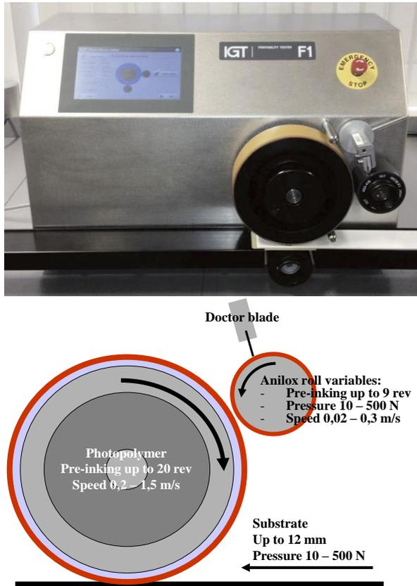
**Fig. 1. IGT F1 Printability Tester Operation.**
