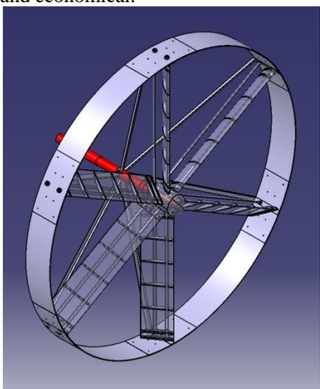
**Fig. 2. Highlighted axle of the rotor**
