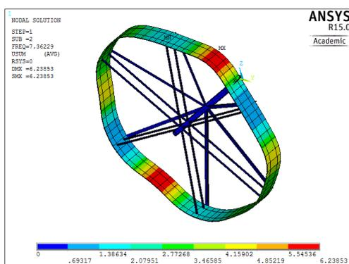
Fig. 14. First mode of vibration – 12 [mm]
