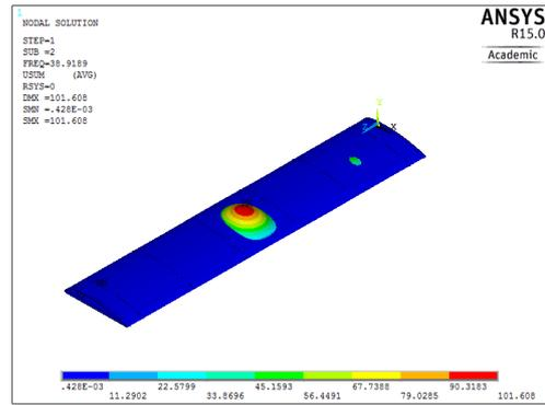
**Fig. 10. First mode of vibration – metallic configuration**
