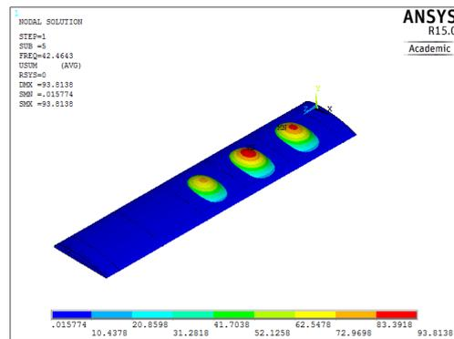
**Fig. 11. Fourth mode of vibration – metallic**
