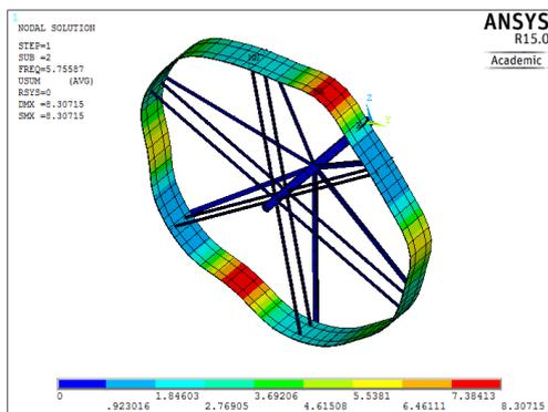
Fig. 12. First mode of vibration – 7 [mm]
