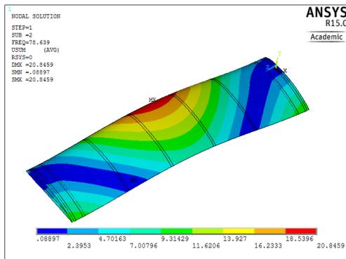
**Fig. 8. First mode of vibration – foam filled**
