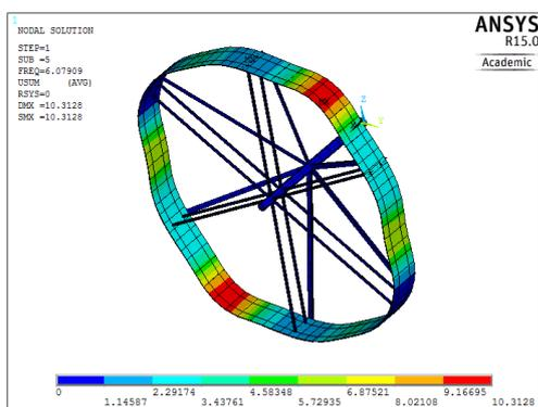
Fig. 13. Fourth mode of vibration – 7 [mm]
